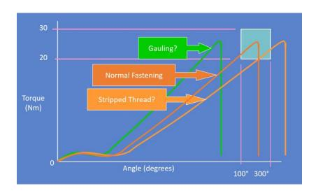
If you are using angle to verify the quality of your joint, the angle reported by the controller/tool should be verified.
