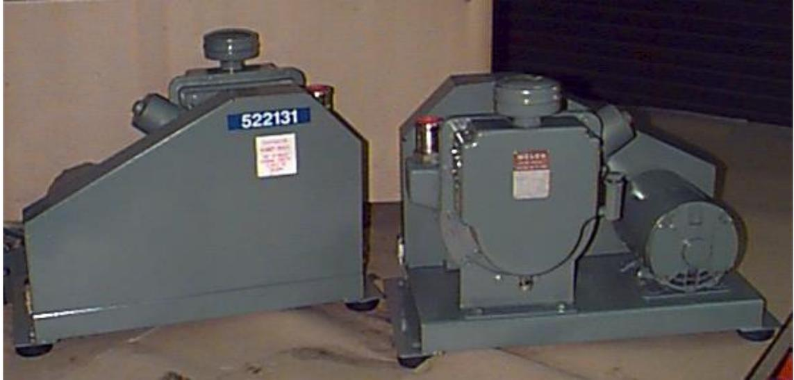
The items pictured are the same units with two views. As you can see there is a pump and electric motor mounted on a pedestal. The pump is driven by two belts. The size of the pumps are dependent upon the amount of vacuum required for the application.
