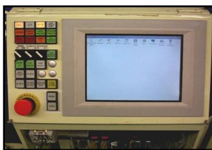
IDEC Monitor Touchscreen Control Panel
