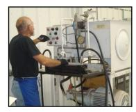
All repaired cylinders are dynamically tested to verify proper operation and leak free performance.
