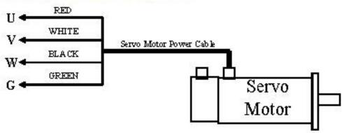
Motor Stator Or Cable Issues Can Cause Many Drive Faults Including "High Or Excessive" Current Errors, Positioning Errors, Intermittent Faults As Well As Many Others.
