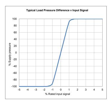
The flow tolerance for standard servovalves is  $\pm 10\%$  of the rated flow at 100% rated input signal.
