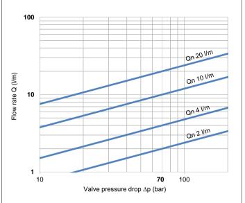
The flow tolerance for standard servovalves is  $\pm 10\%$  of the rated flow at 100% rated input signal.
