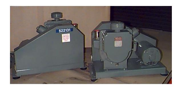
The items pictured are the same units with two views. As you can see there is a pump and electric motor mounted on a pedestal. The pump is driven by two belts. The size of the pumps are dependent upon the amount of vacuum required for the application.
