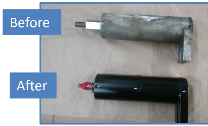
Centerline cylinders with old seals
