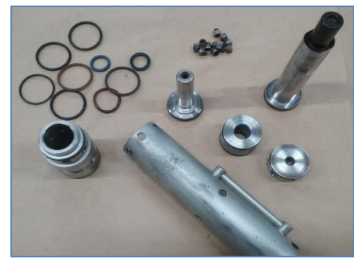
Centerline cylinders with old seals
