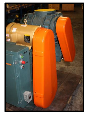
Model 1736 is a combination of a Stokes 212 Pump and a Stokes 607 Booster Pump Assembly
