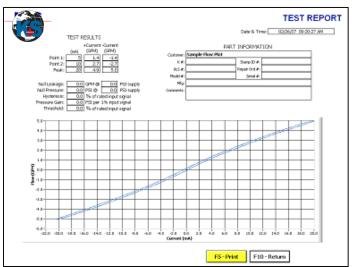
K+S Services has the capability to repair most Bosch Rexroth valves seen in the market place. These Proportional and Servo valves are fully tested and documented with computerized flow plot generation.
