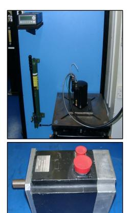
K+S Services can repair and fully load test several series of Moog AC Servo Motors. Below are some examples of the models that we have repaired:
