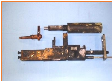
Weld Gun AFTER Rebuild
