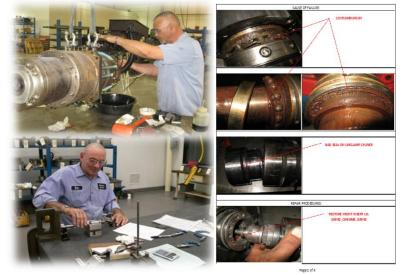
All aspects of the spindle are monitored for critical run out with vibration & temperature measured at maximum RPM's. Videos are taken for each spindle during final test.
