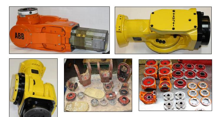
Each wrist is completely disassembled. All components are cleaned and inspected. Each item is carefully prepped for reassembly. Each completed wrist assembly is fully tested prior to return to our customers.
