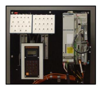
The Indramat DKS is an intelligent digital ac servo compact controller that can be set up for multiple configurations depending on the plug-in cards installed. Our test stand is set up for the most common of these which includes a DLC01.1-FW control interface, a DEA4.1 system I/O, and a DEA 5.1 extended I/O. A dedicated set of I/O control boxes were built and an Indramat CTA keypad is used for programming. Drive status and parameters can be observed with the RS232 computer interface.
