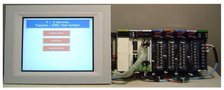
K+S has the ability to repair the Toyopuc PLC3JD system with an integrated IDEC video touch panel. This system has special I/O and touch screen programs written for it to ensure complete system testing.
