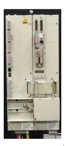
This is the Siemens 611 Universal AC servo drive system. This system can effectively test 6SN1145 infeed or power supply modules, 6SN1123 servo power modules and 6SN1118 control cards. In addition, This Siemens "universal" servo system can be adapted to dynamically test most all Siemens AC servo & spindle motors on the market today!
