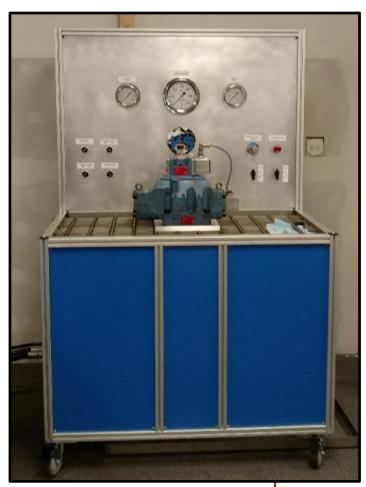
This valve test stand is specifically designed for Proportional Valves and can also support Servo Valves. The Test Stand includes key components, such as:
