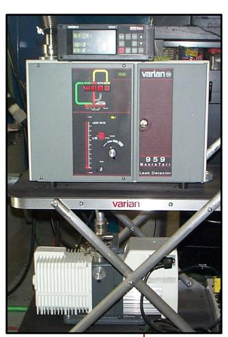
K+S Services utilizes a number of various pieces of testing equipment to fully test all vacuum products. We use the Varian 959 Porta-Test Leak Detector which has a minimum detectable signal / sensitivity of 2 x 10-8 atm cc/sec (helium) sniffing mode to detect leaks in accordance with AVS standard 2.1.
