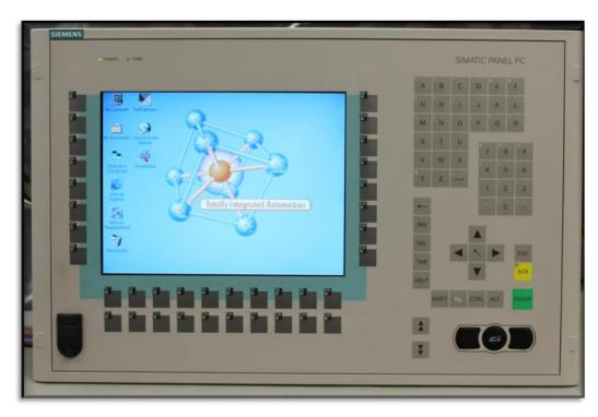
K+ S Services, Inc. has the ability to repair and test the Siemens Simatic Panel PC line such as the PC670 shown here. Utilizing OEM specific software, we can test the complete unit including the computer, touchscreen, and further enhances our current Simatic test and repair capabilities.
