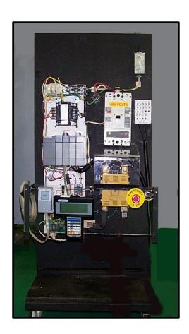
The completion of the Medar Medweld 3005 test stand system is integrated into the Allen Bradley SLC500 PLC system and is used throughout the industry as a resistive weld control. The Medweld 3005 system is used as a single weld control (as pictured) or may run up 16 weld controls through the \*Mednet Networking system. The system contains the following components
