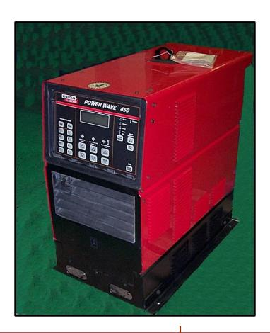
The INVERTEC Power Wave is a high performance, digitally controlled, synergic welding system used in conjunction with a robotic wire feed system.
