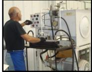
All repaired cylinders are dynamically tested to verify proper operation and leak free performance.
