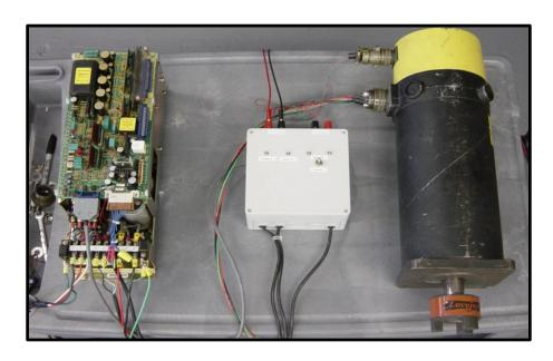
This FANUC velocity control unit (VCU) is a single axis servo control module. This unit is diagnostic tested by a closed loop run / load test with a Fanuc DC servo motor. Also, all VCU I/O points are tested with this fixture. The Fanuc VCU can be either single or dual drive types. Other series units are as listed:
