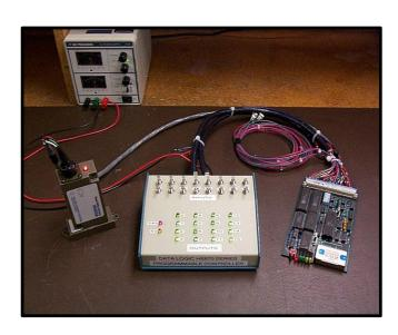
K+S Services has the ability for full power dynamic testing for the Data Logic HS870 Series Programmable Controller. The test system is capable of fully exercising all inputs, outputs, communication, and antenna functions.
