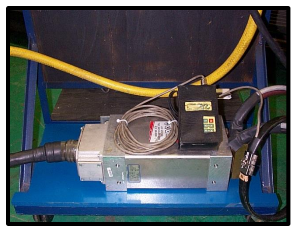
60KVA Weld Transformer
